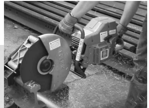
Kwik Kut wheel shown on Racine Ultra Kut II rail saw
