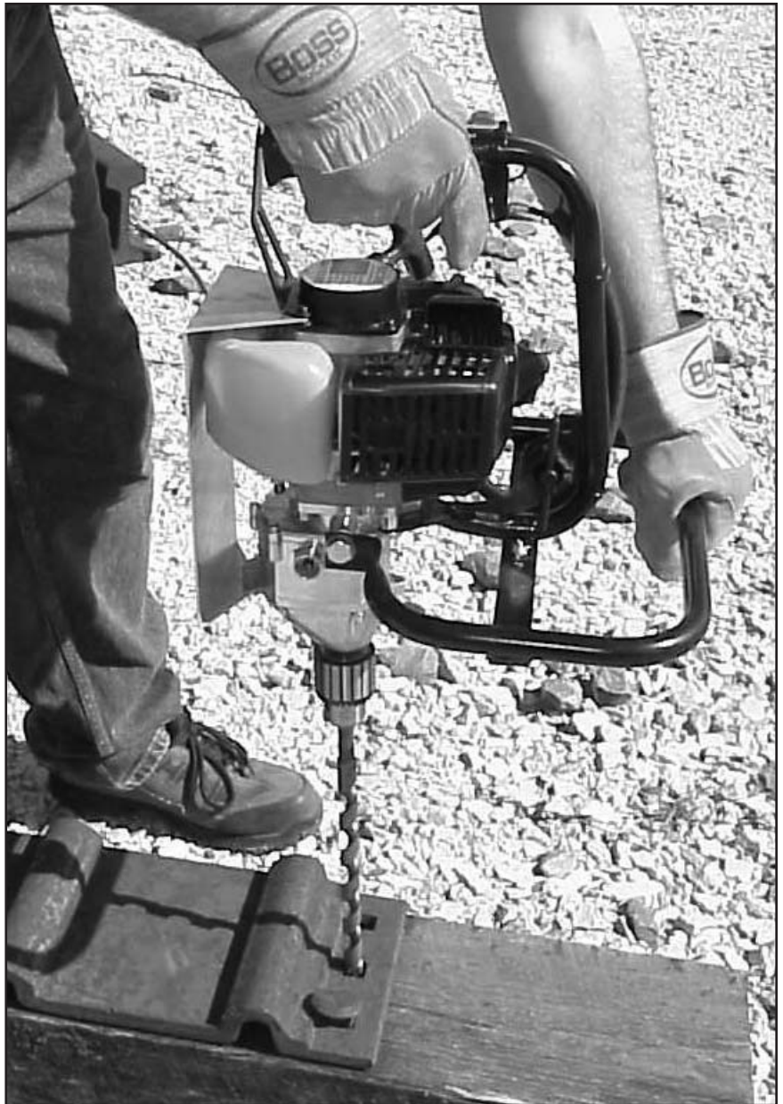
The Racine Gasoline Tie Drill is designed to pre-drill holes in wood ties for lag screws, bridge timber screws and crossing projects.
