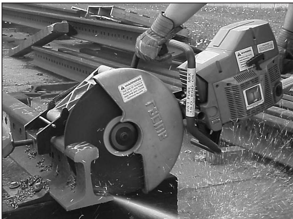
Lightweight 44 lb power unit easily attaches to clamp and arm assembly.
