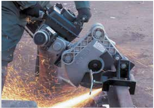
Racine Abrasive Wheel shown on Racine Trak Kut II rail saw.
