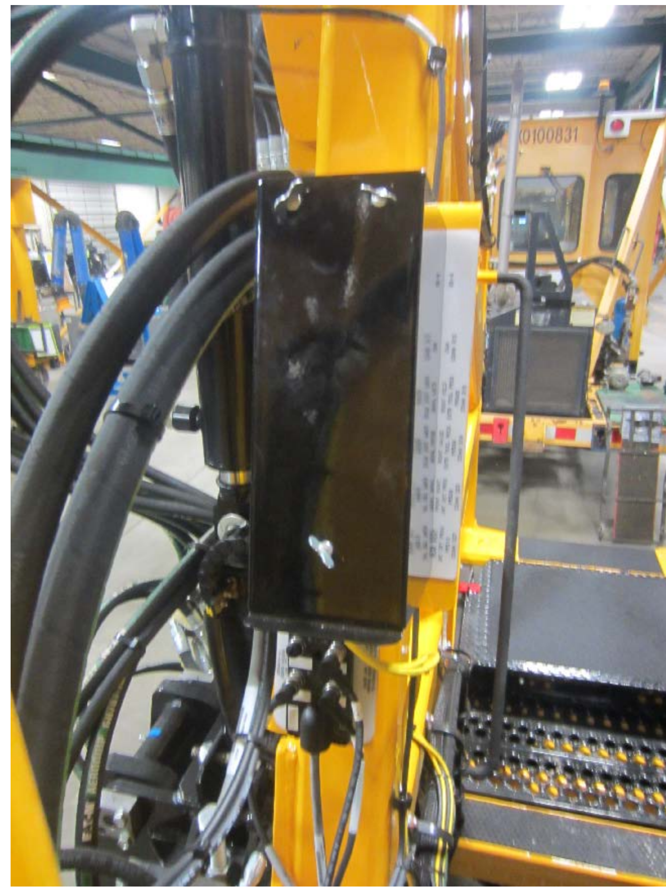
COVER ALIGNED WITH MURR BLOCK 1/4 TURN THUMB LOCK
