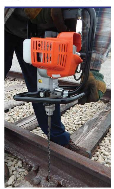
The Racine Gasoline Tie Drill is designed to pre-drill holes in wood ties for lag screws, bridge timber screws and crossing projects.
