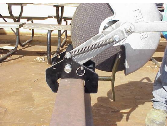
Rail Side Cutting with Operator's Position Adjacent to Clamp Tensioning Screw Stop Pin is inserted on operator's side.
