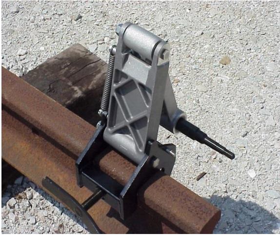
Rail Clamp Installed
