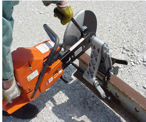
Mounting the Ultra Kut II Saw
