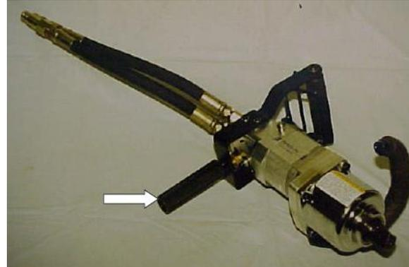
An additional handle kit can be added to the impact wrench to position a handle directly across from the main operating handle.
