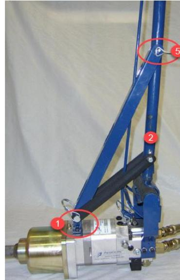
5. Pull back on the handle to align the upper holes in the handle pole and the holes in brace arm.
