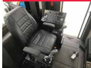
Operator station with ergonomic seat and joystick controls.
