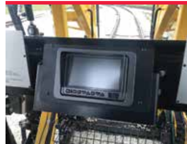
Camera screen to view the field clips during apply / remove operation.
