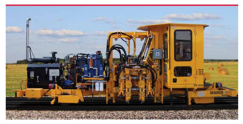
The Racine Rail Tie Straightener is designed to work out of face to straighten concrete ties in full crib at up to 5-6 ties per minute.
