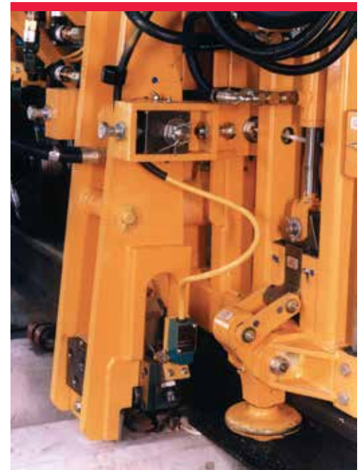
Close-up of workhead prior to clip application.
