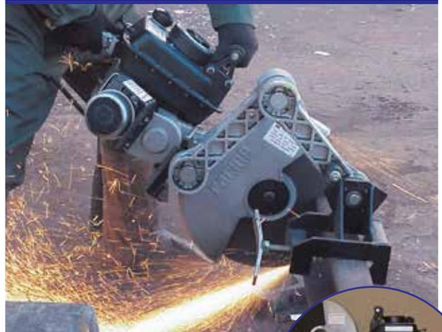
The Racine Trak Kut II Turn-around Rail Saw is designed for cutting rail using a 16" abrasive wheel.
