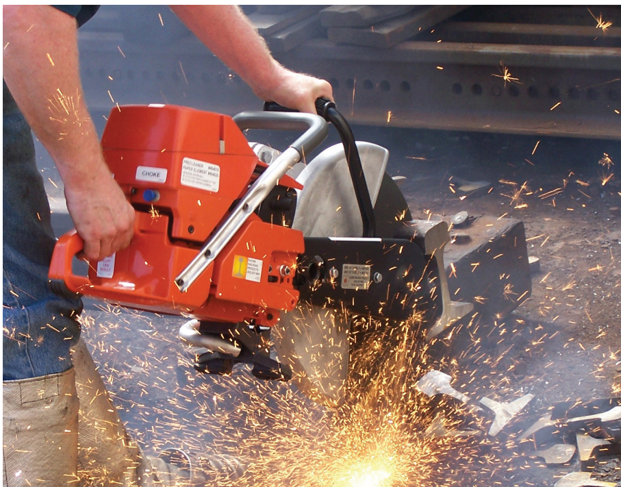
Lightweight 44 lb power unit easily attaches to clamp and arm assembly.
